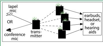
The receivers get their FM signal via a preselected ADA FM frequency broadcast by the portable transmitter. The transmitter (which looks very much like the receivers) picks up sound from one of two different microphones. One mic is a small desktop conference microphone attached to the transmitter for group meetings like Bible Bookworms. You will usually notice the transmitter and conference mic placed somewhere in the center of the group.
